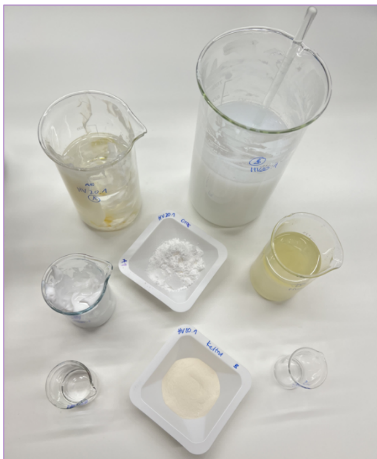
Figure 11 Raw materials for emulsions; especially raw materials of the oil phase such as waxes, emulsifiers and co-emulsifiers offer potential for better energy efficiency.
